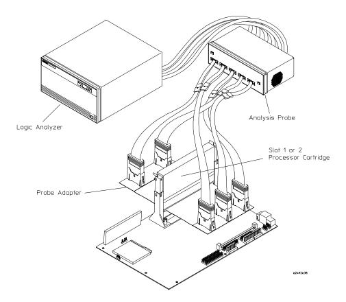
This Installation Guide explains how to install Hewlett-Packard's probe adapter for slot 1 & 2 Intel Pentium II processor cartridges. The probe adapter provides a quick and reliable connection from a slot 1 or 2 processor to the HP E2487A/C Analysis Probe. The analysis probe then connects to your HP logic analyzer for state analysis.
